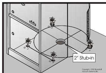
**\*Front bolts must be flush with top of nut for product tank clearance. Bolt may need to be trimmed.**
