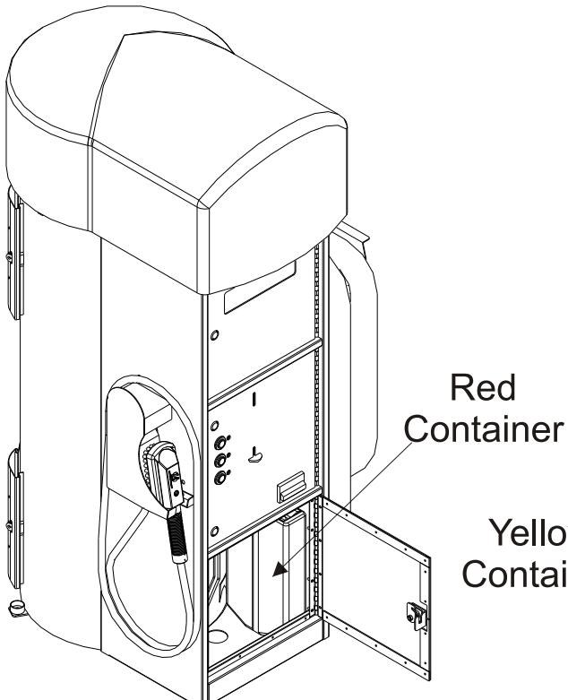
● Remove the product containers from the bottom front cabinet door by unscrewing the container brace from the far right container (container 3). Then remove containers 1&2 which are still attached to the container brace. Now you can access the mounting bolts.
