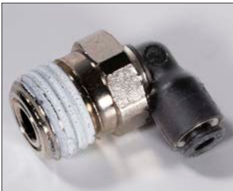
Part # 5030020 Fitting, 1/8 tube x 1/4 NPT elbow
